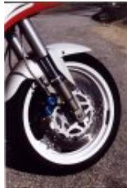
**(8) Close up of the '93 FZR1000 forks (Race Tech springs and Gold Valves). FZR rim and fender and the R1 calipers/ Goodridge lines/ Galfer pads grabbing 320mm rotors. Matched up with MEZ 1 130/60/17 and you have unbeatable stopping power.**
