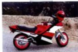
**(10)This is my next changover. Of course you know it's fantasy/ workahead. YZF 750 swingarm modification and rim (going for 180/17 tire). Underslung rear caliper. Ohlins rear shock from '92 FJ. Removable passenger mounts. Adapted Graves rearsets. YZF750 forks with Race Tech Gold Valves(if needed) Traxxion Dynamics springs. R1 calipers and of course the 320's. This time I'll go with red powdercoating. and Since I have a pristine '87 upper fairing, This paint scheme looks likely.**
